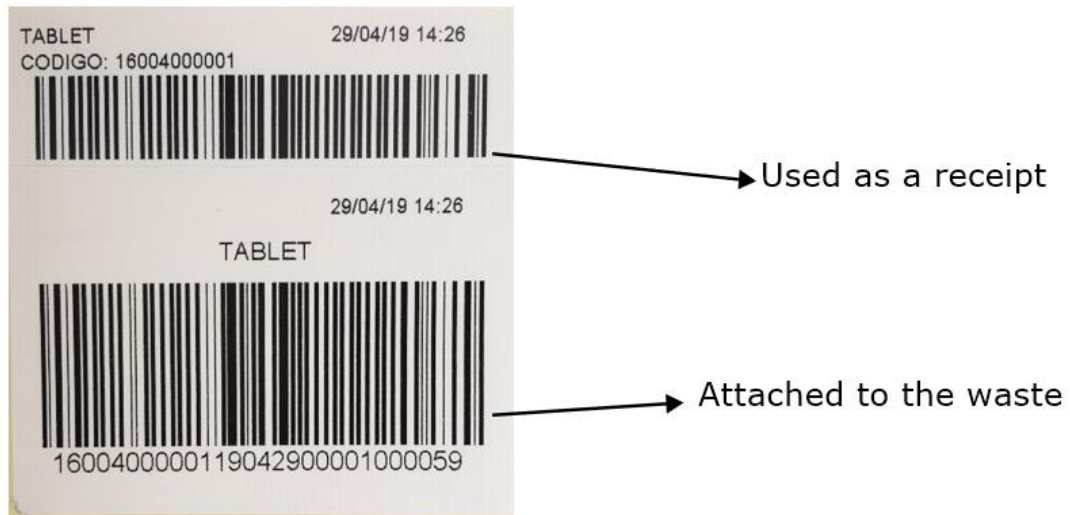
Figure 12 Barcode labels printed by the Intelligent bin
