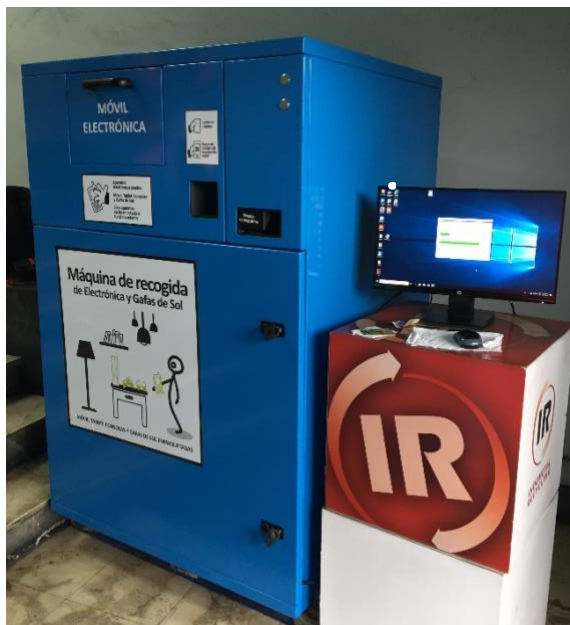
a) Intelligent bin with control unit software installed
