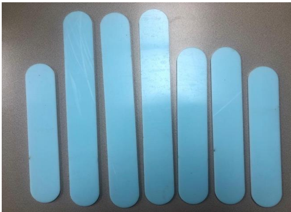
Figure 3.12 Plastic pieces (first prototype) of the housing
