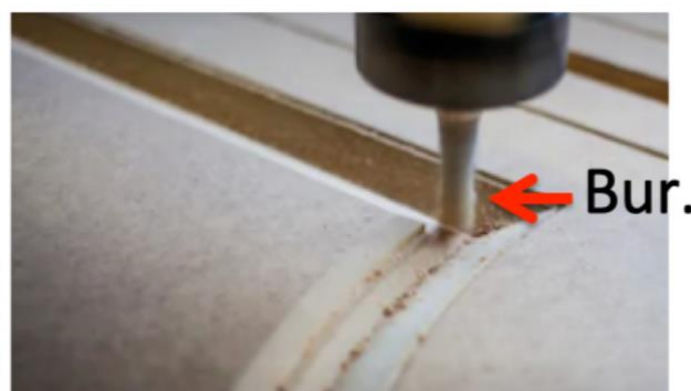
Figure 3.20 Using bur to cut the wood piece
