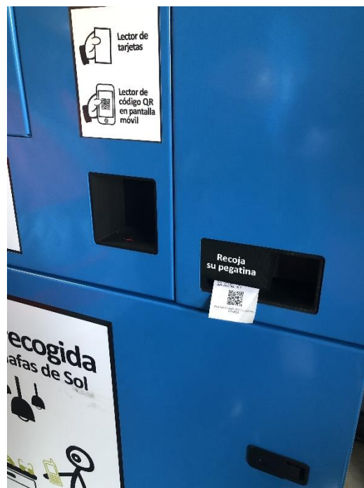
Figure 3: Picture of the intelligent bin with a barcode sticker used for CEBM collaborative recycling
